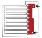
NOTE: If your case has a cover over the PCI screws, also remove the cover.
