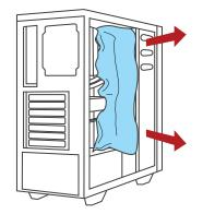
Carefully and gently remove the protective packing foam from inside the system
