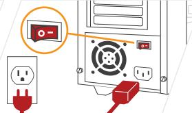
Plug-in the power cord and switch on the power supply before hitting the power button
