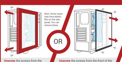
**Unscrew** the screws from the left side panel and remove panel
