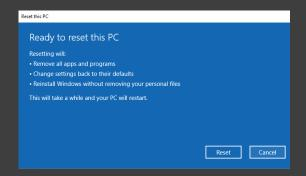
5. Click "Reset" button to confirm and start system reset process
