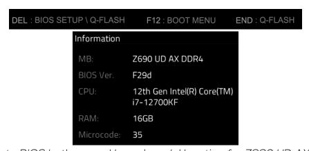
Gigabyte BIOS hotkeys and board model location for Z690 UD AX DDR4
