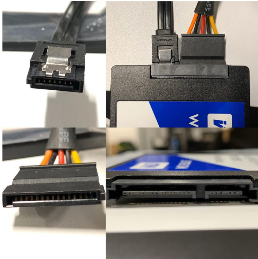
Figure 2 - SATA drive with power and data connectors
