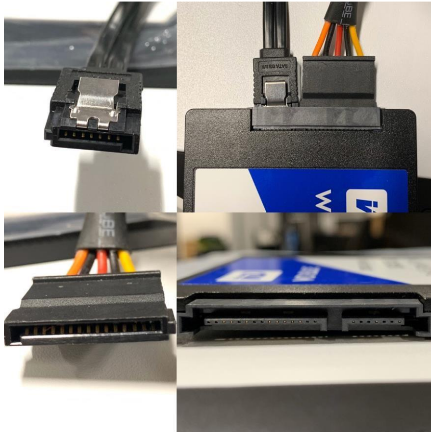
Figure 2 - SATA drive with power and data connectors
