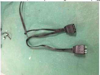
• Make sure your pins are aligned properly. Non-addressable lighting is protected so it will just not turn on if plugged in backwards. Addressable lighting will burn out if plugged in reverse. Most
