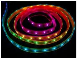
• Non-Addressable – This refers to analog LEDs in which the entire strip is always the same color at any given time. They run off 12 Volts and are not compatible with addressable LEDs. They will use a 4 pin connection the majority of the time.
