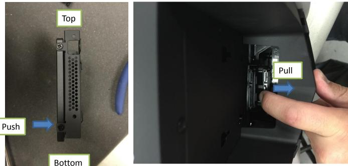
When using both SATA ports up front, it is highly recommended to not use the metal carrier, as it will become much more difficult to remove due to double the friction. The plugs for the SSD are semi flexible so you might need to pull the outer plug towards the front of the case to get it to line up with the SSD
