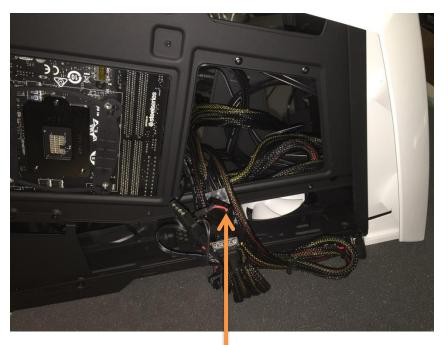
Zip tie the 24 and 8 pin down to the bottom of the cable bar. Don't catch any of the headers in this Next start pulling the other cables through. Bundle unused cables.
